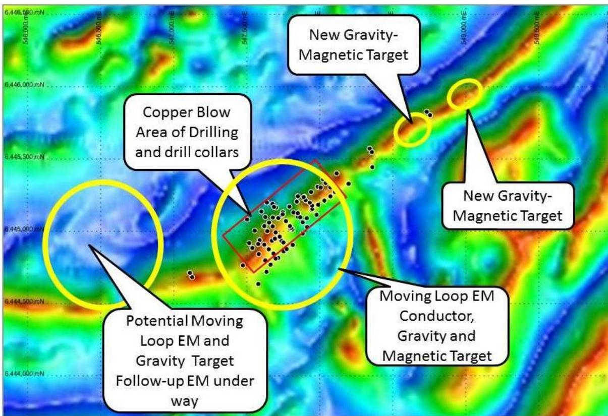
**Figure 4** Summary diagram of new geophysical targets
