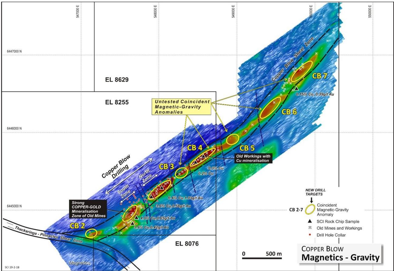
Figure 1 Magnetic image of the Copper Blow trend. Diagram shows the main area of drilling represented in Figure 2 (below), including the North and South Zones.
