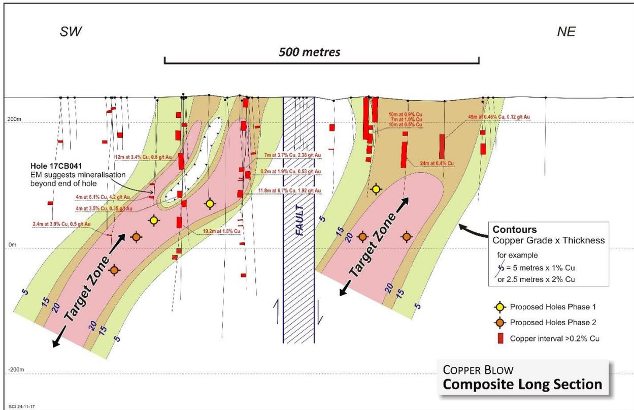
**Figure 2** Long Section (from Figure 1). Composite diagram of >0.2% copper and grade x downhole thickness contours. Data suggests southerly or southwesterly plunge to mineralisation both north and south of the Central Fault. Hole 17CB041 hosts an interpreted downhole EM response indicating mineralisation off the end of the hole.
