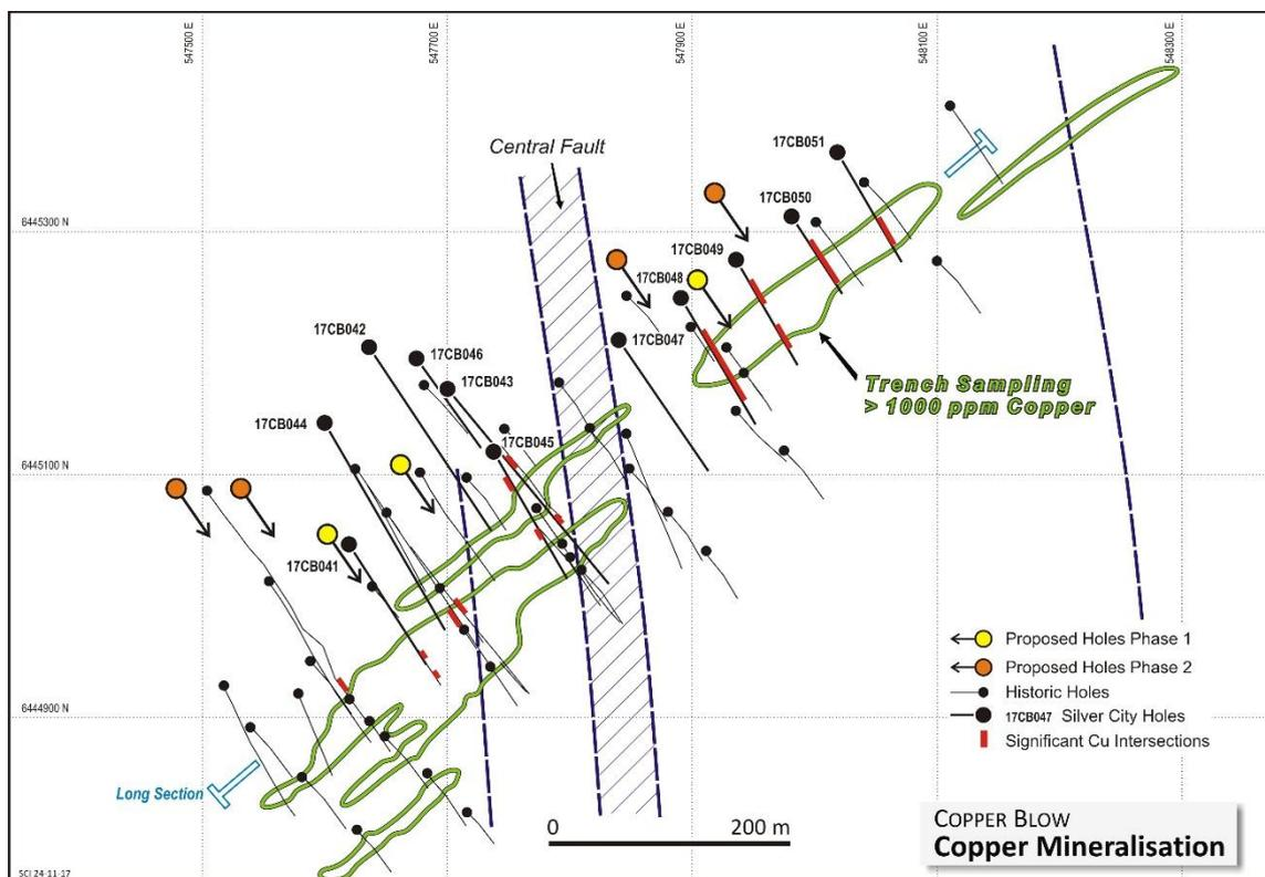
**Figure 1** Copper Blow drill hole locations with significant mineralisation represented as red bars on drill traces. Central Fault separates high grade and deeper mineralisation in the south from broad zones of lower grade in the north.
